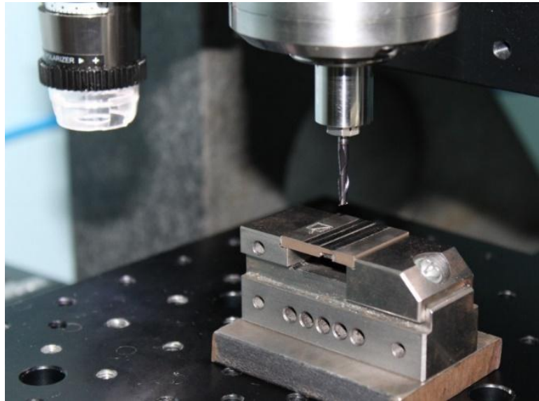
Fig. 1: High Speed Spindle for High Speed Micro Milling Operation
